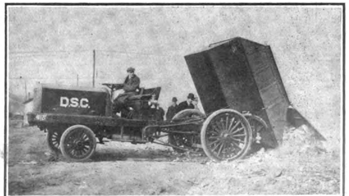
Showing the dumping body raised to perpendicular as it deposits its load
